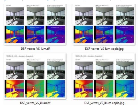
Figure 123: Comparison of natural lighting between using different glass for the windows (Radiance).
