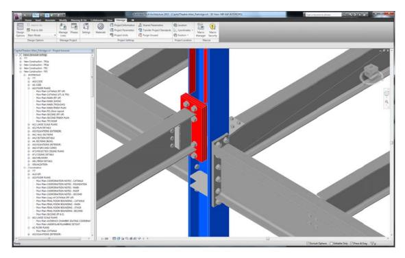
Figure 131: Detail of structural steel work that was incorporated into the Revit Structure model.
