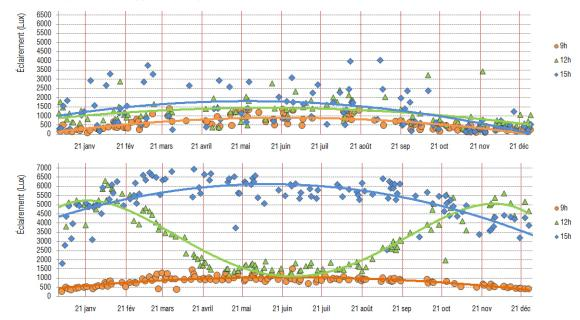
Figure 121: Graphics generated with Radiance: comparison between a cloudy (above) and a sunny (below) sky illumination on an office (S-W).
