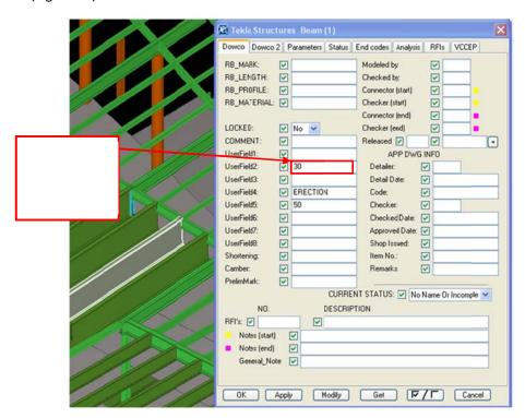
Figure 79: Division numbers were assigned to the steel in Tekla Structures to support exporting to Navisworks Timeliner for 4D modeling of steel and concrete work.
