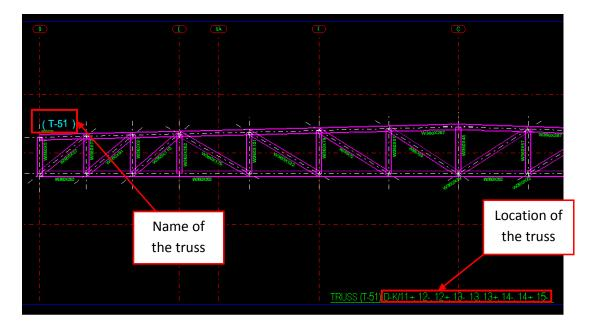
Figure 71: Example of a truss elevation showing the name of the truss and where it is located. The truss name and location appeared automatically on drawings using specific attributes added to the model.
