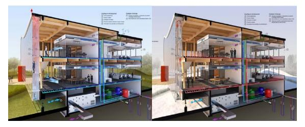
Figure 111: Ventilation and cooling during the Summer (left); Ventilation and heating during the Winter (right)
