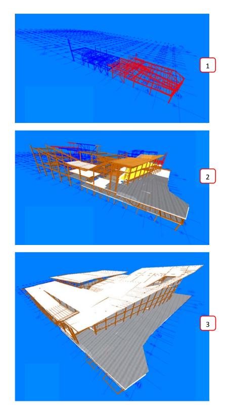
Figure 80: 4D visualization showing: (1) two zones of steel erected; (2) approximately half the steel structure and concrete pours constructed; (3) the completion of the steel and concrete structure.
