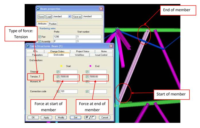
Figure 68: Forces added to certain members in the model in the 'Beam Properties' dialogue box.
