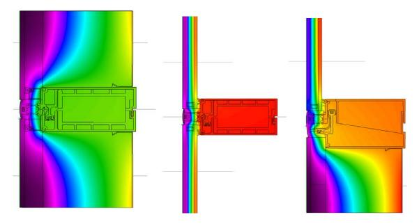
Figure 125: Graphics generated from Therm – presenting heat transfer around a window with different colors presenting temperature variations.
