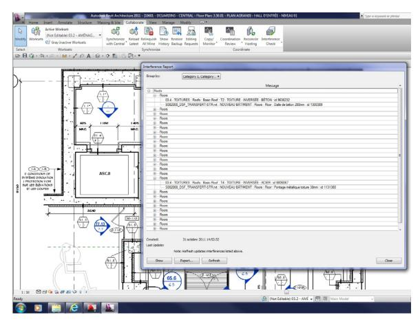
Figure 128: Interference report for Clash Detection from Revit.
