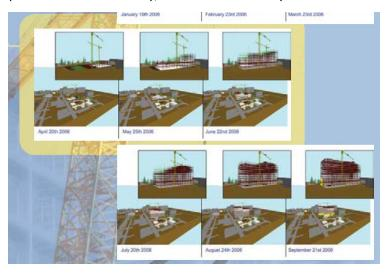
Figure 45: 4D visualization enabled instantaneous feedback on the schedule (Mortenson, 2009)
