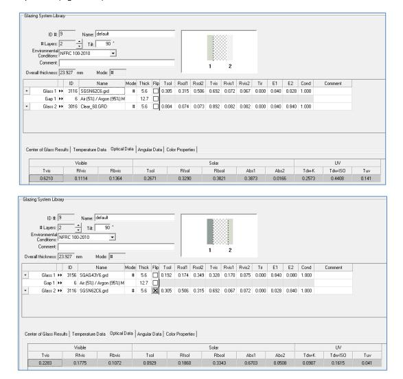
Figure 124: Properties of a window glazing: tables generated with the Window.
