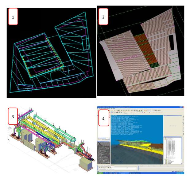
Figure 66: Multiple BIM models created by the (1) Architect, (2) Structural Engineer, (3) Mechanical Trade and (4) Contractor.
