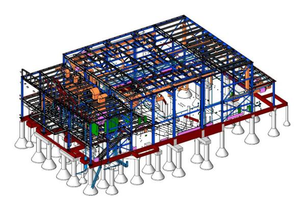
Figure 133: Tekla Model (integrated into BIM) that allows easy visual auditing of all design components
