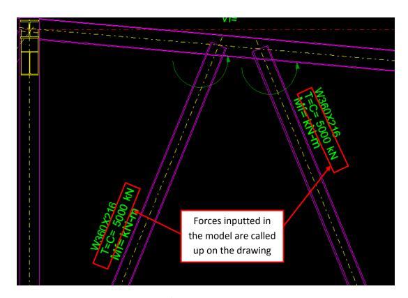
Figure 69: Elevation drawing showing how the forces were added automatically on each member.
