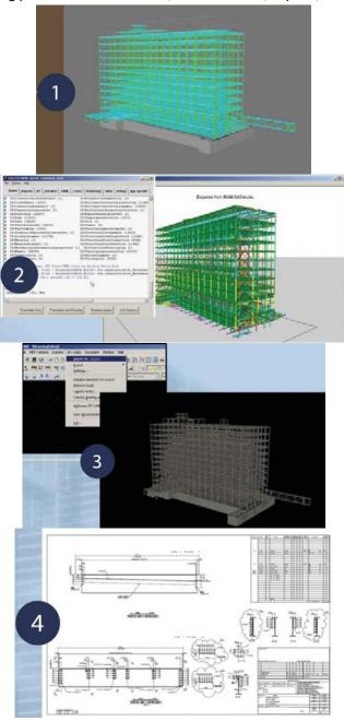
Figure 43: Creation of steel shop drawings: 1) structural steel analysis model, 2-3) steel detailer/fabricator model, 4) structural steel shop drawings (Mortenson, 2009)
