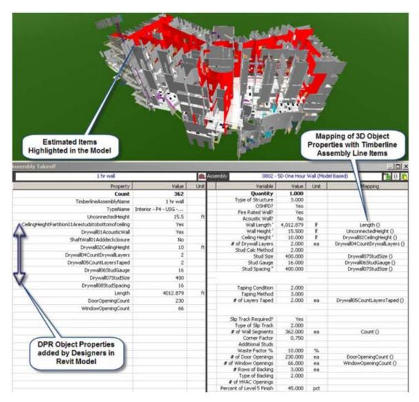
Figure 28: Mapping the 3D model to Cost Assembly in Timberline through Innovaya (Tiwari et al. 2009)
