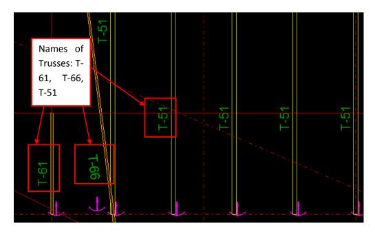
Figure 72: Example of a truss schedule which is a plan drawing showing the locations of steel trusses. The truss names are added automatically.
