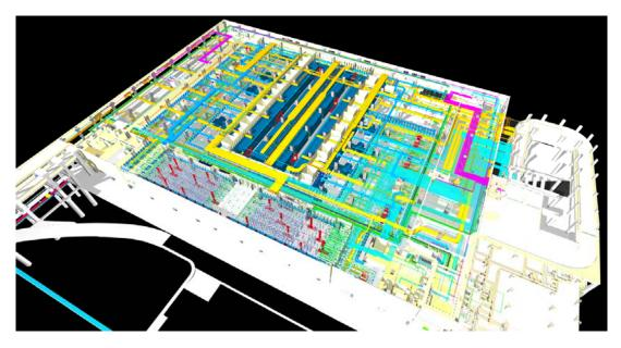
Figure 52: Combined BIM model for clash detection (floor view in NavisWorks).
