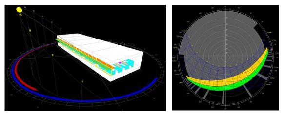
Figure 120: Left - Study of shading and reflecting devices: the model; Right - occultation from the shading (green) and effect of the tablet (yellow).
