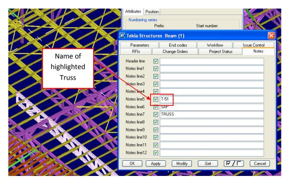
Figure 70: Names were given to trusses in the model that could then be called up automatically on a truss elevation and truss schedule.
