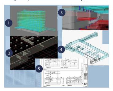
Figure 44: Creation of assembly instructions for concrete construction (Mortenson, 2009, images modified)
