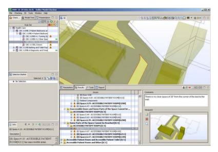
Figure 26: Checking the model for accessibility and other ADA code compliance using Solibri Model Checker (Khemlani 2009)
