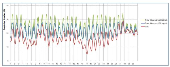
Figure 119: Temperature of the surface of the curtain window glazing (oriented to the South) with and without exterior pergola.
