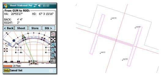
Figure 132: Trimble used to verify anchor bolts prior to finalization of base plates.
