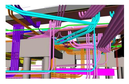
Figure 23: Underground Model (Ghafari Associates, accessed on Oct. 2011)
