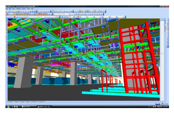
Figure 53: Combined BIM model: warehouse (virtual walkthrough in NavisWorks).
