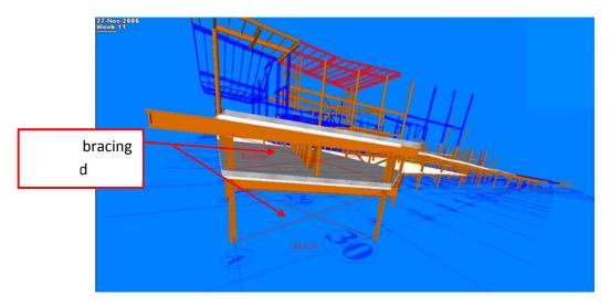
Figure 81: Engineer steps through the 4D model to identify where temporary lateral bracing is required during construction.
