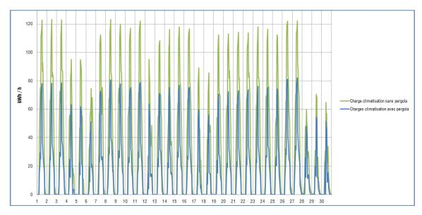
Figure 118: Cooling energy consumption in the cafeteria in June with (dark) and without (light) exterior pergola
