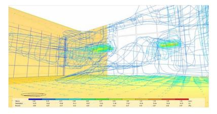
Figure 126: Spatial representation of speed and temperature of air near an open window: speed vectors (above); speed contours (below)
