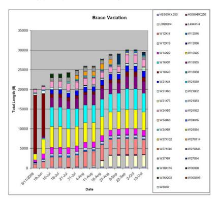
Figure 27: The quantity take-off and trending for structural bracing automatically derived from the model at different stages of the design (Khemlani 2009)
